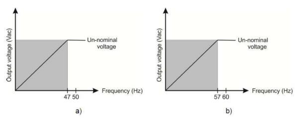
Under frequency "knee": a) 50 Hz system, b) 60 Hz system
