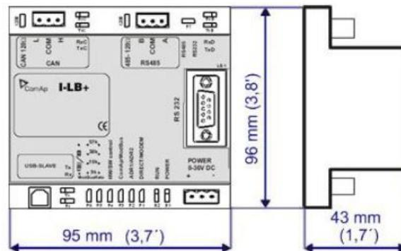
Unit is 35 mm DIN rail mounted.
