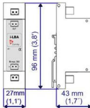
**Note:** Unit is 35 mm DIN rail mounted.
