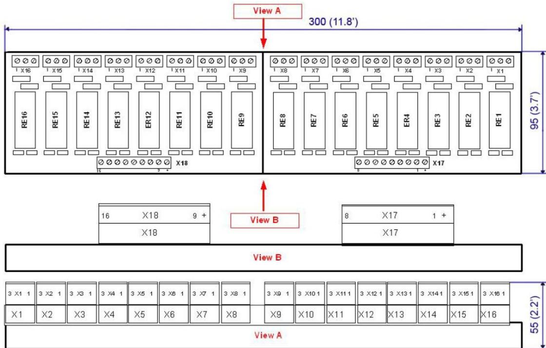
Image 4.2 Unit is 35 mm DIN rail mounted.
