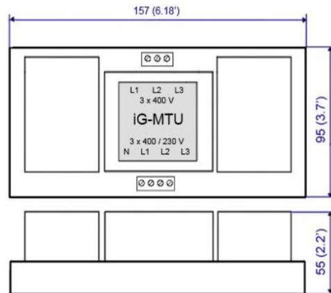
Unit is 35 mm DIN rail mounted.
