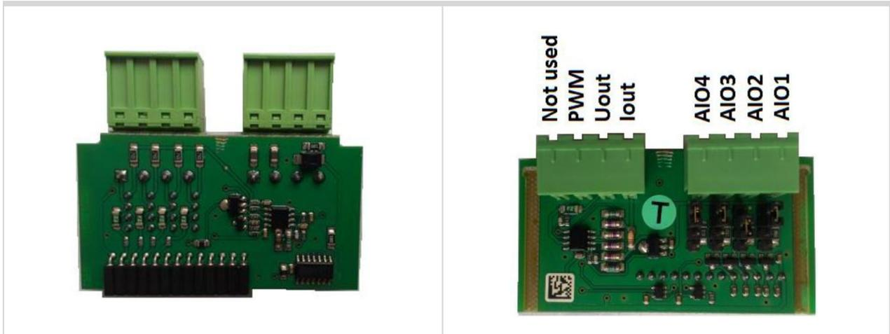
Type of analog input is selectable by jumper. Each analog input has own line of jumper position. The top position (closest to green connector on the pic above) is for resistive input, central position for voltage input and lowest position is for current input.
