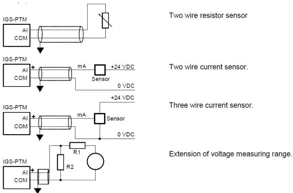
**Note:** It is not necessary to connect analog inputs COM terminal to negative power supply.
