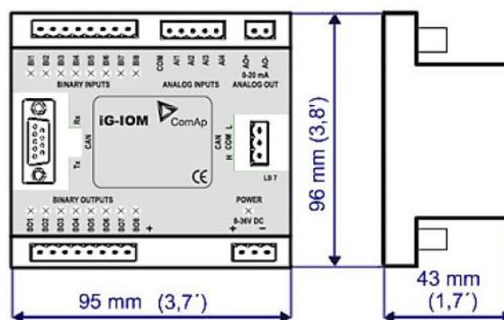
**Note:** Unit is 35 mm DIN rail mounted.
