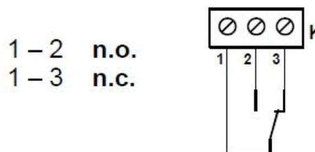
Image 4.3 Relay-connector connection
