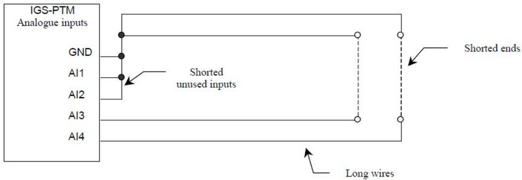
**Note:** Maximum resistance of two leads (from IGS-PTM to sensor and back) can be 20 Ω. Otherwise the compensation fails. Unused analog inputs must be shorted at the IGS-PTM.
