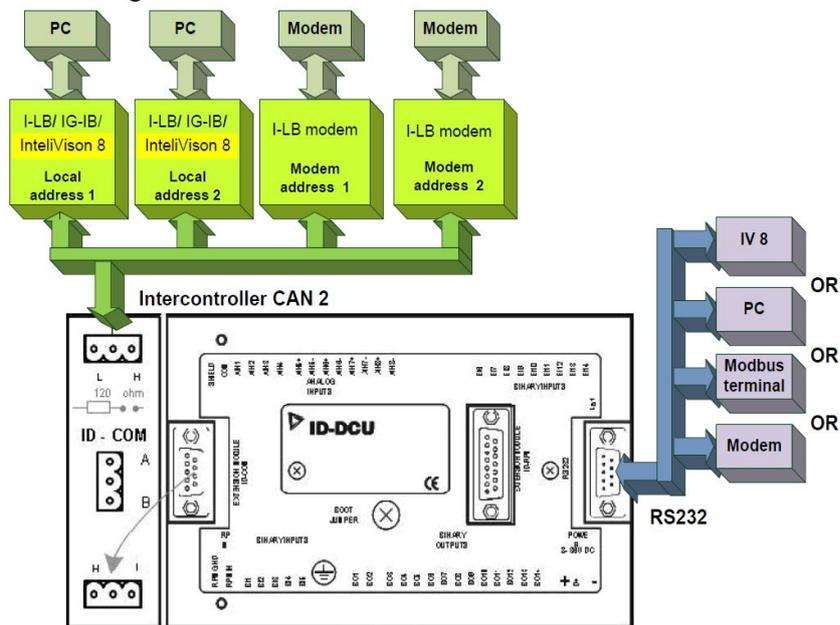
Image 9.5 IntelliDrive DCU wiring
