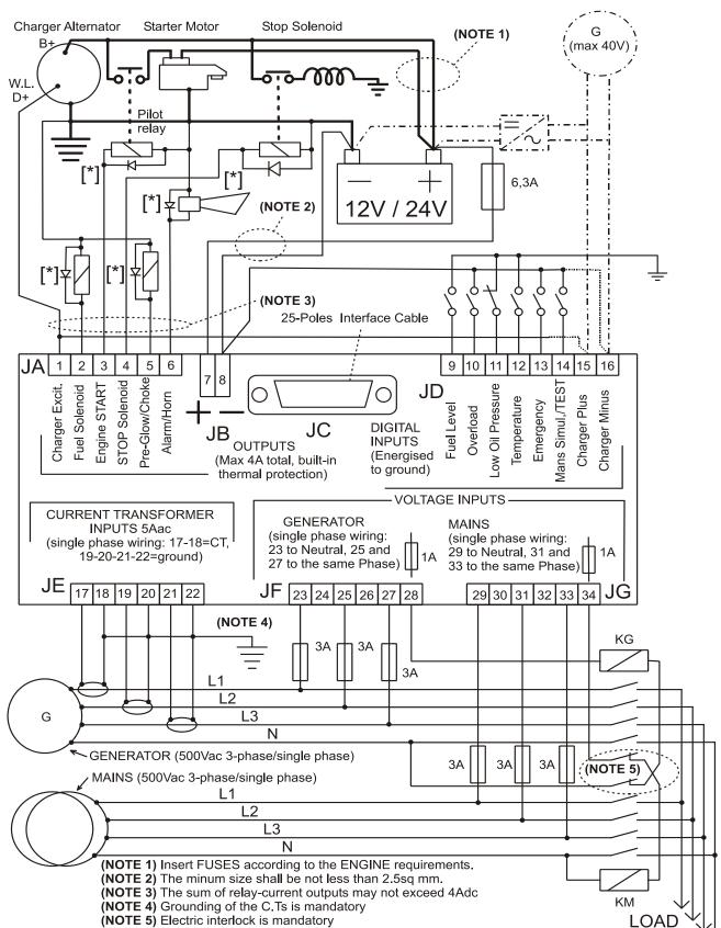
[\*] Suppress relays at source using flywell diodes or suppression devices
